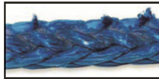
Melting or Glazing Area will be Stiff
