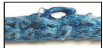
Rope Strands Reduced 25%* from Abrasion
