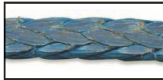
Compression Slight Sheen Is Visible**
