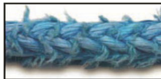
Rope Diameter Reduced 25%* from Abrasion
